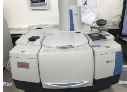
Figure 9: L'instrument ATR (NICOLET iS50 ABX FT-IR - Thermo-SCIENTIFIC
