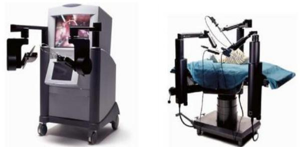
Figure 6: Robot chirurgical Zeus [44]
