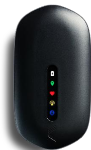
Figure 4 : Dispositif Catapult Vector S7
