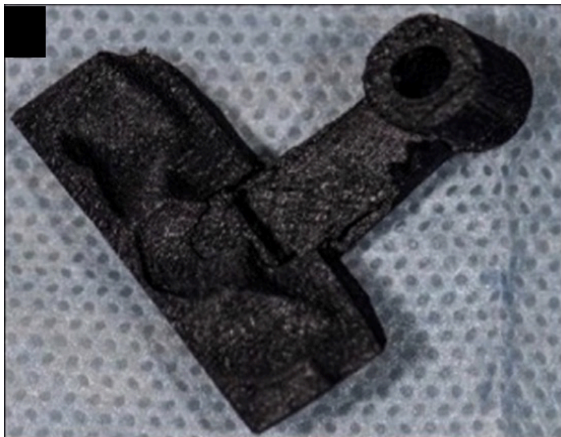
Figure 22 – Guide chirurgical en polylactide [44].
