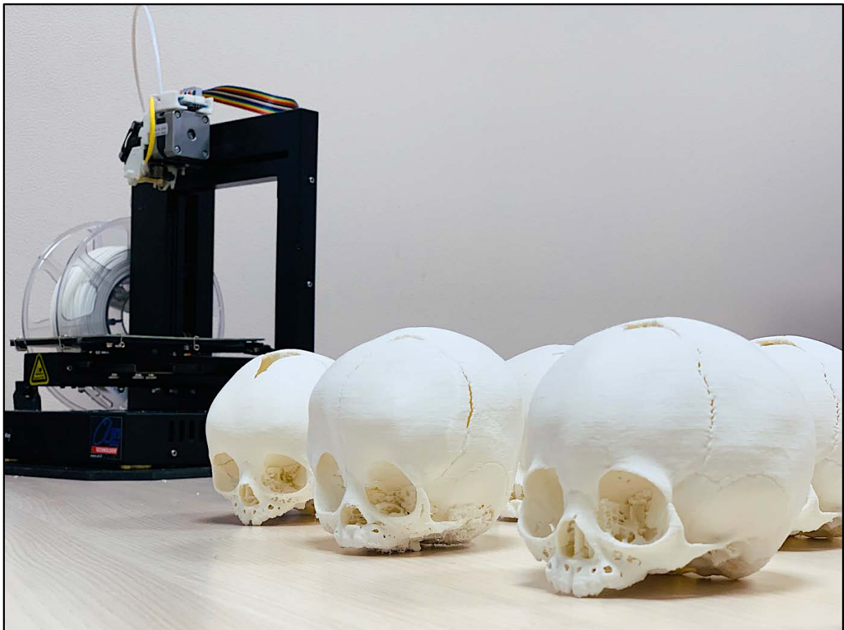
Figure 1. Set of 3D-printed models representing three of the four types of craniosynostosis.
