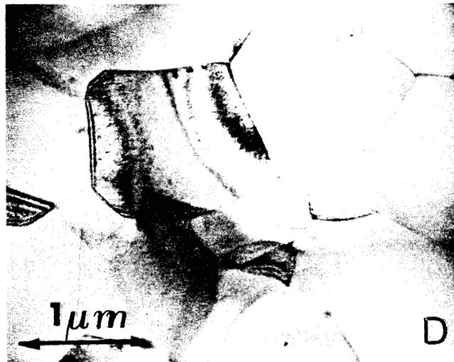
1100°C,  $\epsilon = 14\%$ ,  $t = 100 \text{ min}$ ,  $\bar{d}_g = 0,9 \mu\text{m}$
