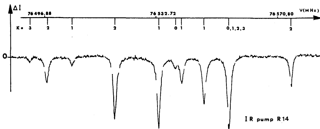
Fig. 3. Variations of intensity observed with the R14 laser line in the microwave spectra and identification of the lines.
