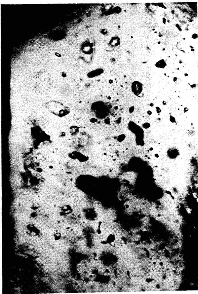
Figure III-1. Photograph of DA-CHANG fluid inclusions.
