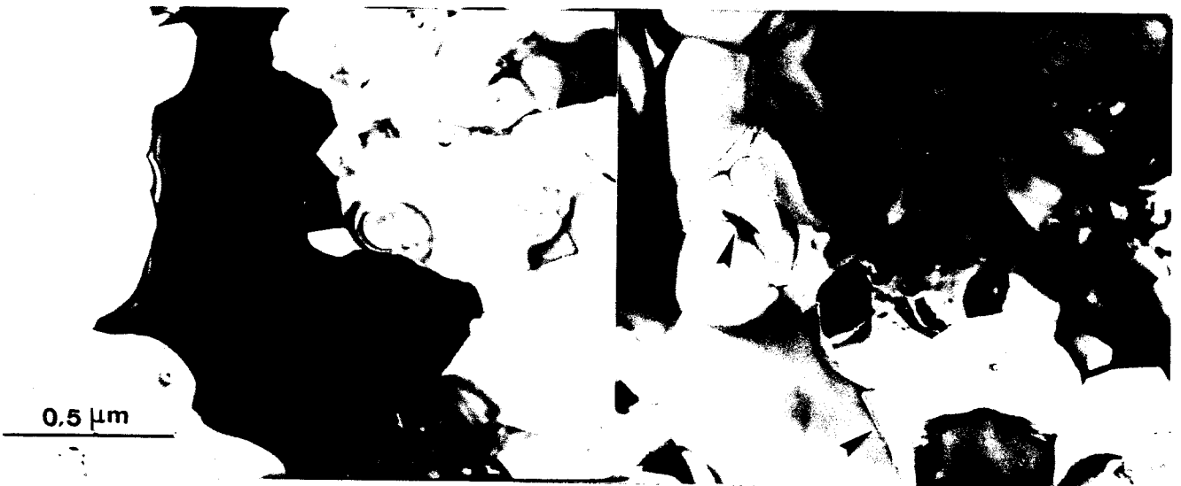
b. Microstructure mixte T = 1400 - 1370 - 1340 - 1300 - 1260^{\circ}\text{C} t = 210 \text{ h}
