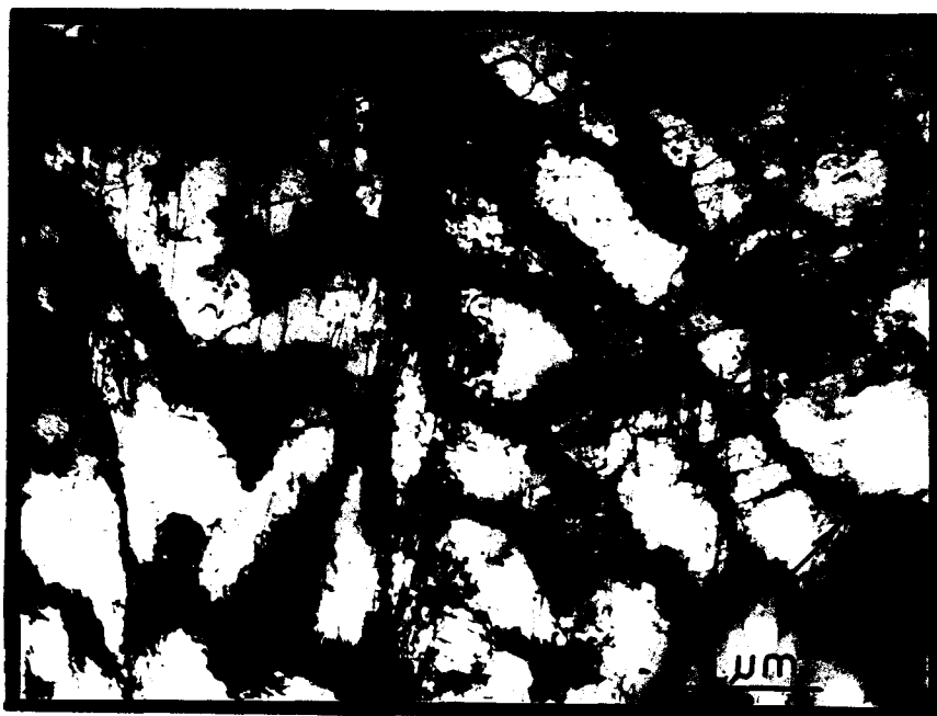
Figure 1.12 : mélange de 2 types d'arrangements \Delta\epsilon_t = 1\% , T = 300K ; N_R = 4\ 500 cycles
