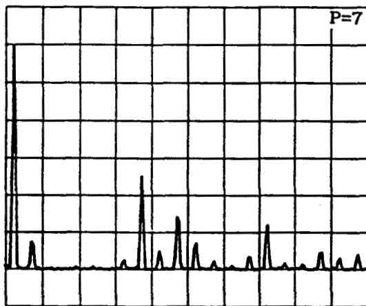
RES1 is result of FOURIER TRANSFORM function. VER: +13.9 V HOR: + 200 Hz
