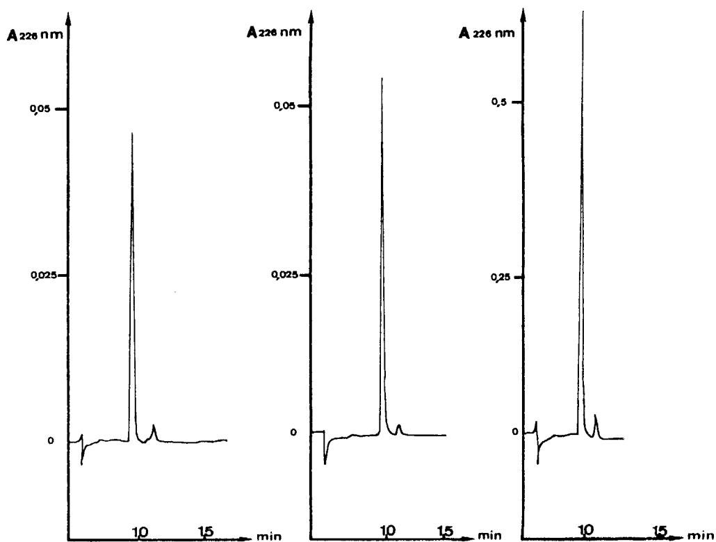
**Figure 4 :** *C18 reversed-phase HPLC on a narobore column of the three AII-like immunoreactive peptides (a, b, c) previously separated on a C18 reversed-phase HPLC column.*
