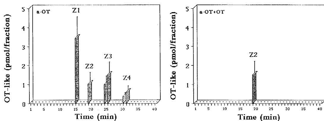
Figure 4- Reversed-phase HPLC elution profile of an extract of 400 brains of *T. tessulatum* at stage 3B.
