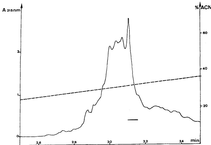
Figure 4 : *C<sub>18</sub> reversed-phase HPLC on a narobore column of the All-like immunoreactive material previously separated on a C<sub>18</sub> reversed-phase HPLC column.*
