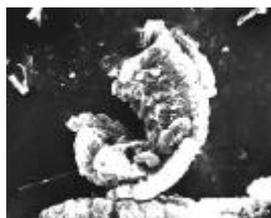
**Fig. 6** : Expanded worm of graphite
