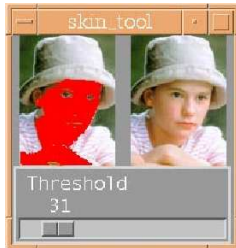
Figure A.1: Snap shot of the tool for segmenting the skin regions of an image. The left image shows the completed manual segmentation with the skin pixels highlighted in red. The right image shows the original image [JR02]
