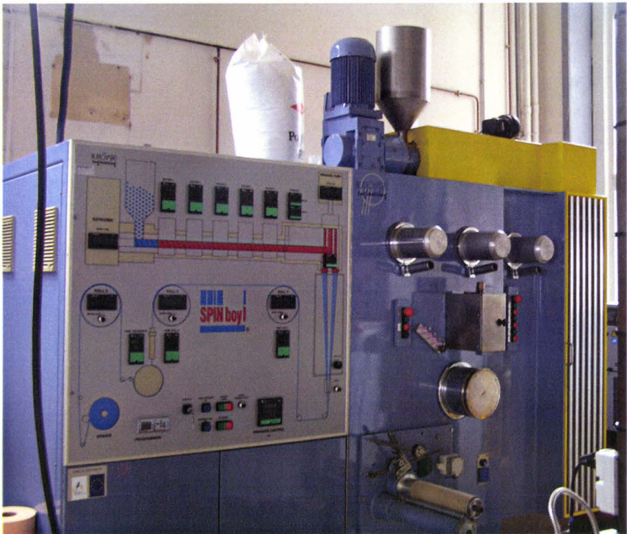
Figure 14. Machine de filage Spinboy I.
