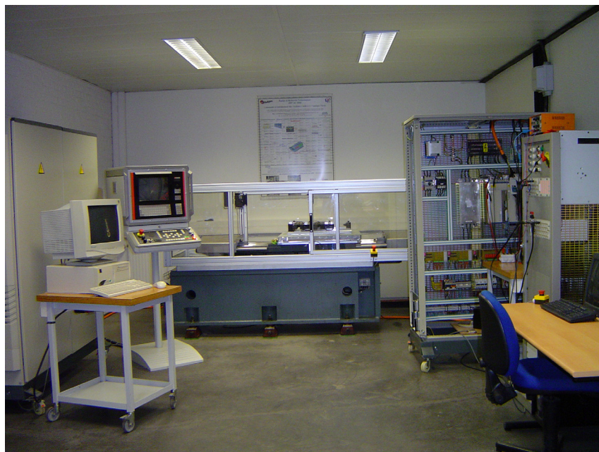
Figure D.4 – Laboratory PMLSM test bench
