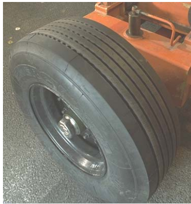
Figure 2.2b : Pneu super single (Michelin 385/65R22.5).
