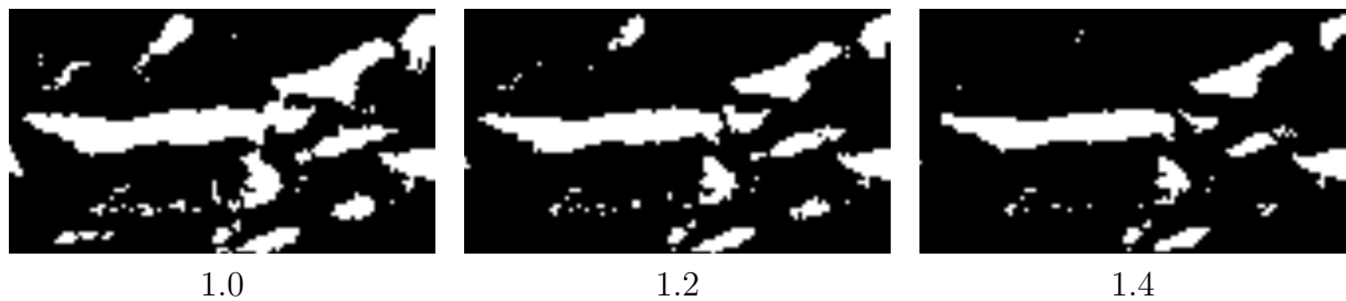
FIG. B.16 – Indicative images after the thresholding procedure with various C_T^v for NVF
