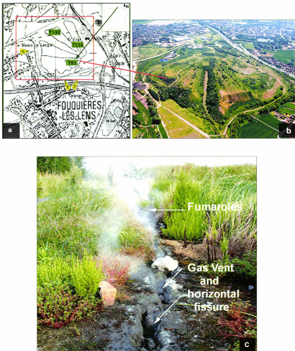
Figure 4. Coal waste heap n°83 Fouquières-les-Lens (Paquette, 2001). (a) Location of the study area 1/25000. (b) Aerial photo of the site, 1/5000° (Paquette, 2001). (c) Surface horizontal fissure and gas vent (35cm wide and 3m long) emission of heat and fumaroles, 2005.
