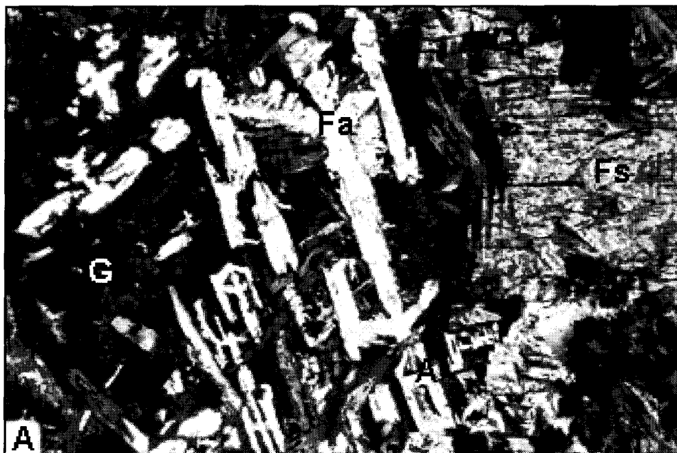
Figure 15A. Transmitted light micrographs x 220 PPL of paralava (sample P1). Typical branching dendritic texture of fayalite (Fa) containing an overgrown skeletal anorthide (A). The gray phase at right top corner is orthoferrosilite (Fs) with inclusions of glass (G) black.
