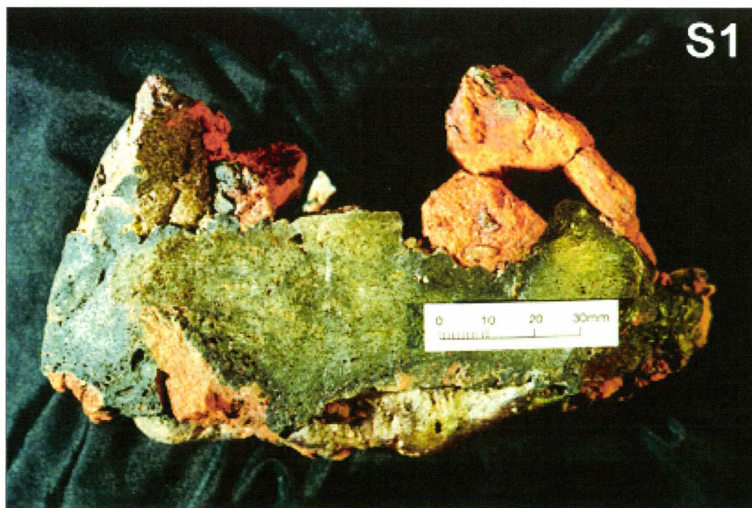
Figure 5. Cut slabs of selected melted iron-rich slags. Note vesicular slaggy material in sample S1 is surrounded by reddish porcellanite.
