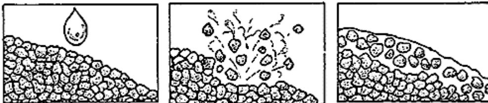
Figure 1.2 Soil particles and aggregates that have been detached by raindrops are transported down the slope by runoff.
